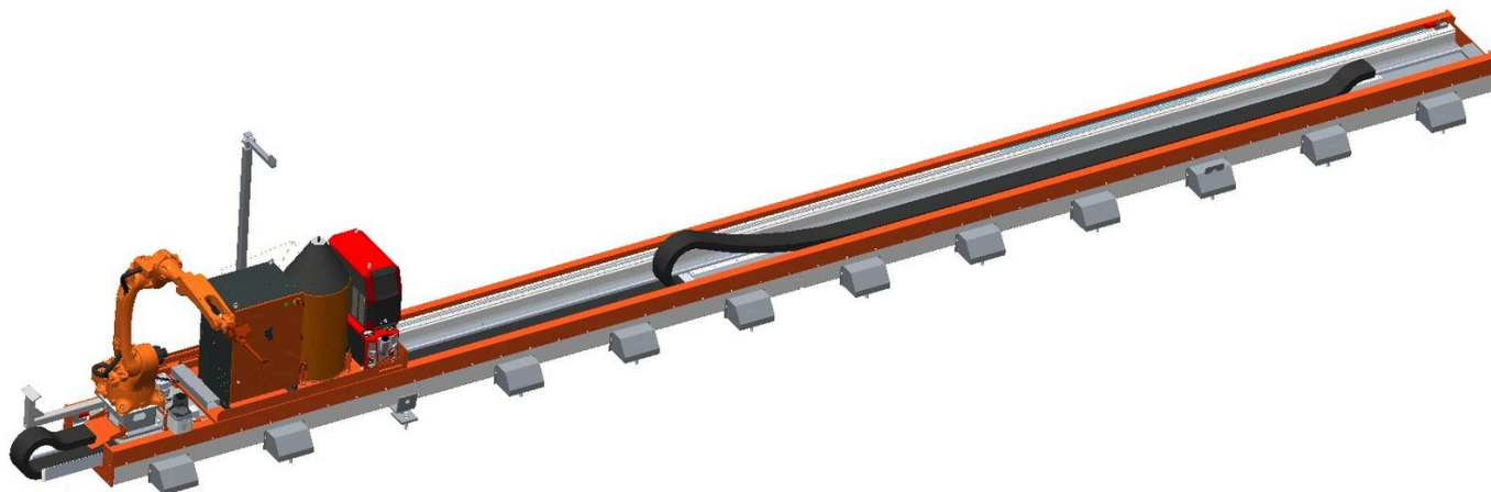
The 7-axis rail-mounted layout.
