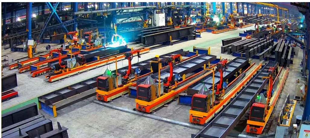
Rail-mounted welding stations in a production hall.
